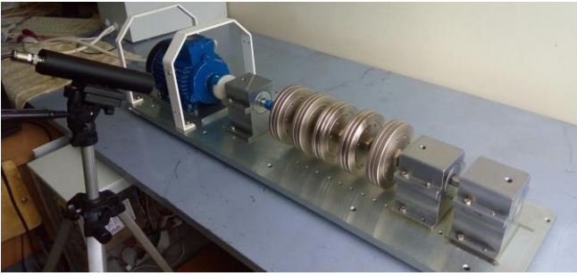
Fig. 4. Test rig for the study of rotor-bearings.
