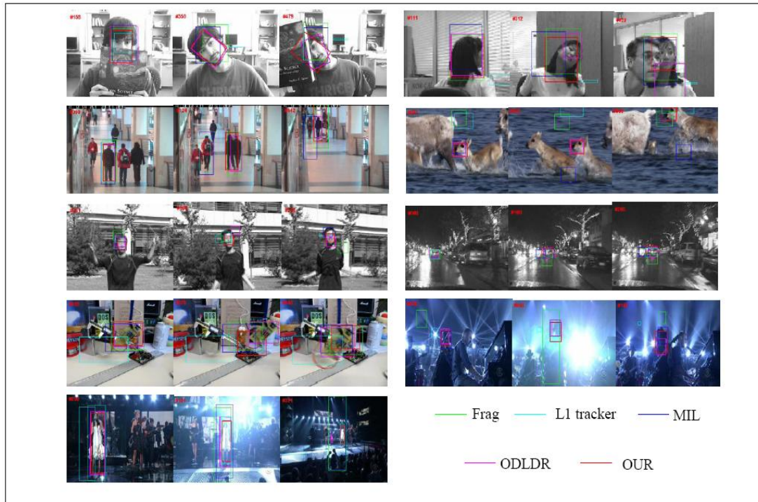
Fig. 3. Sample tracking results of evaluated algorithm on nine challenging image sequences.
